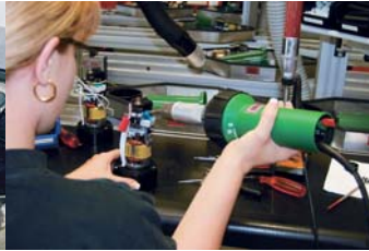
Shrinking a solder sleeve with TRIAC PID.
