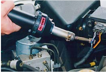
HOT JET S with spoon sieve reflector used to shrink solder sleeves.
