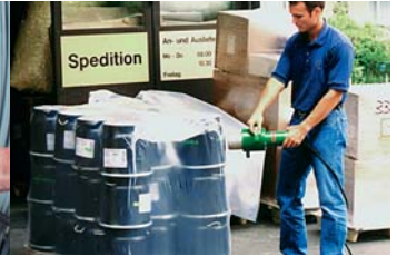
Flameless shrink-wrapping of pallets and bulky goods with the FORTE S3. This allows work to be carried out in enclosed spaces.
